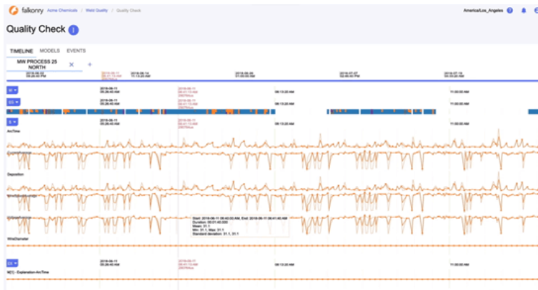
Workbench's Quality Check screen displaying data points over time to help operators identify patterns (Source: Falkonry )
