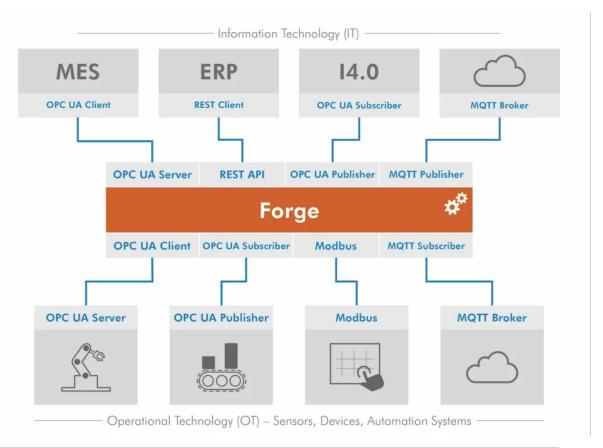
Prosys' OPC-UA Forge enables OT and IT integration by performing data acquisition, data harmonization, and cloud connectivity at the edge. (Source: <u>Prosys OPC</u>)
