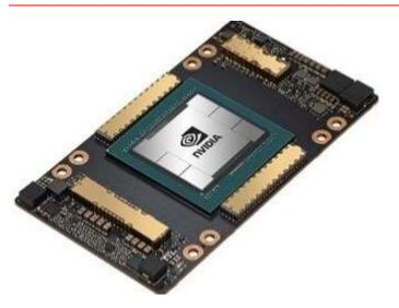
**NVIDIA A100,** the company's flagship GPU for data centers (source: <u>NVIDIA</u>)
